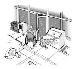
Exterior accessible routes begin at site arrival points, such as accessible parking spaces and the public sidewalk, and may include elements such as curb ramps, walks and ramps. Platform lifts may be used where permitted by the CBC.<sup>10</sup>
